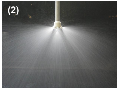
(2) Adaptor with 7 full cone spray nozzles
