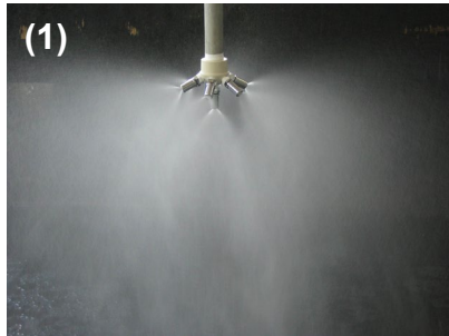
(1) Adaptor with 7 hollow cone spray nozzles
